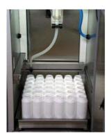
16 x 2.9L 12 x 2.9L + 1 x 12L 5 x 6.4 L 4 x 12 L 36 x 1L as well as composites of various sizes
